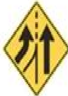
Added Lane sign
