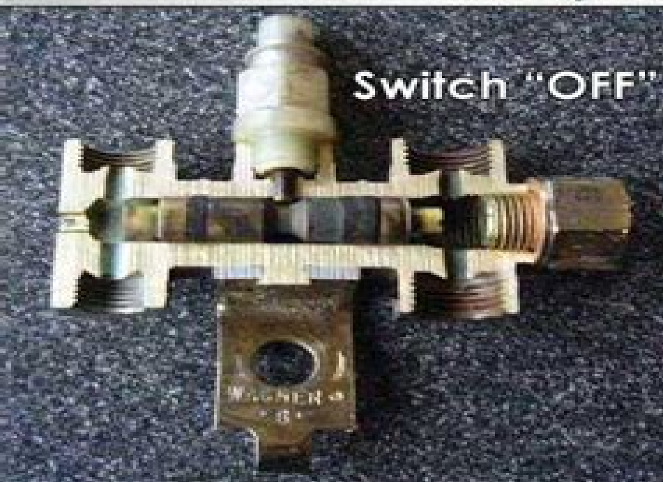
Brake Pressure Differential Valve (NOT a proportioning valve!)
