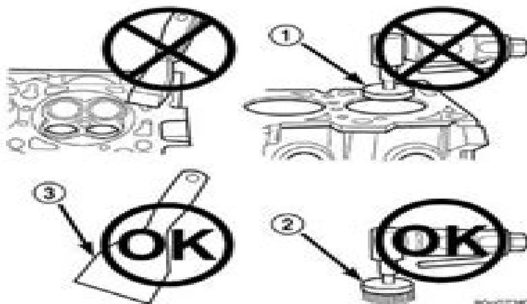
**Fig. 1: Proper Tool Usage For Surface Preparation**
