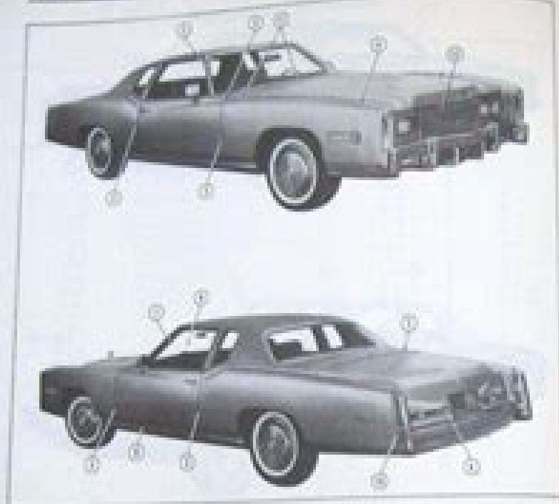
Fig. 11-2 Rear Body Tolerances — Eldorado
