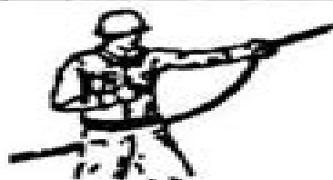
RETRACT BOOM (TELESCOPING BOOMS) ONE FIST THUMB POINTING OUTWARD AND HEEL OF FIST TAP FINGERS CHEST
