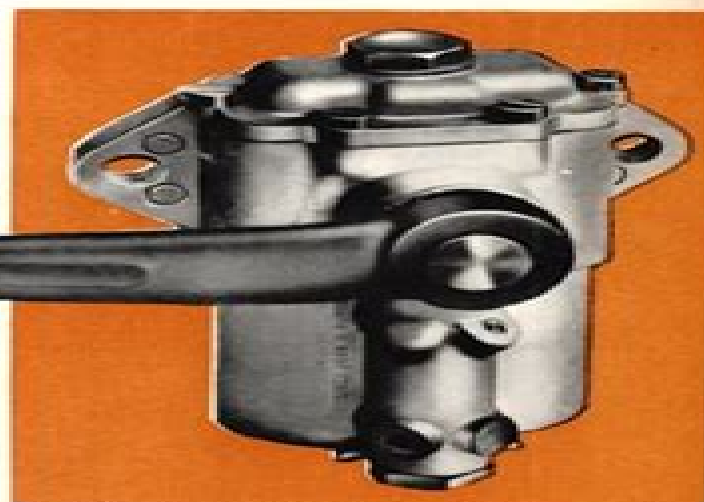
A well-finished exterior is a feature of the Armstrong shock absorber. The cylinder bores have no detachable plugs and no external joints are subject to high pressure, hence no leakage is likely to occur.
