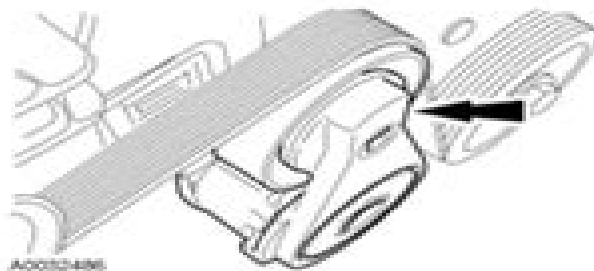
Fig. 14: Locating Accessory Drive Belt Tensioner Courtesy of FORD MOTOR CO.
