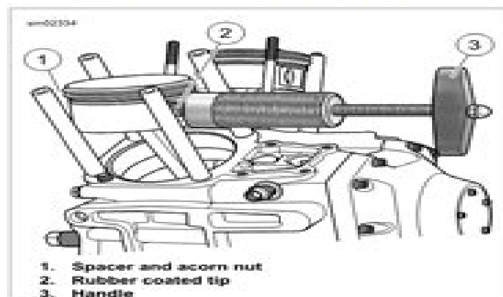
Figure 3-29. Piston Pin Remover (Part No. HD-42320-A)
