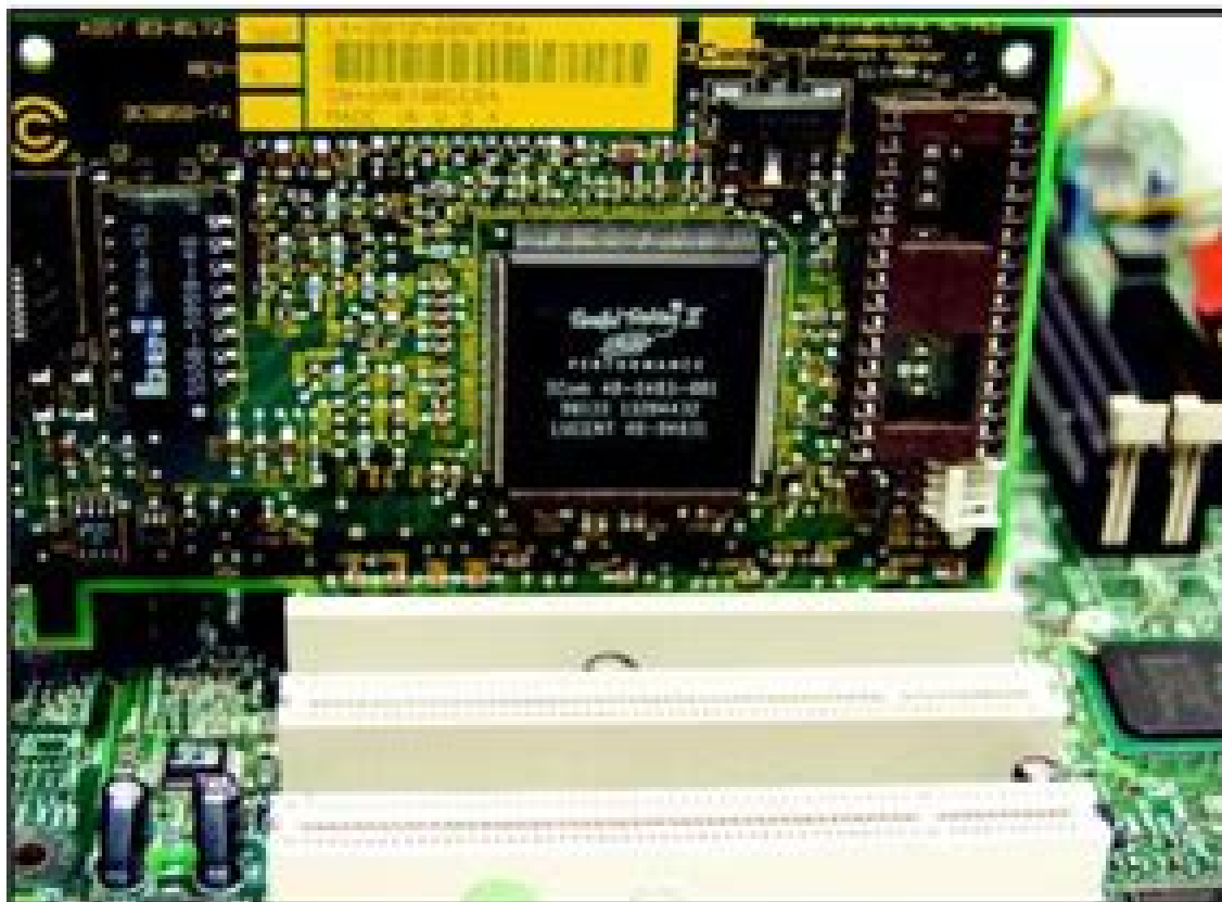
Figure 6-10 A properly inserted NIC
