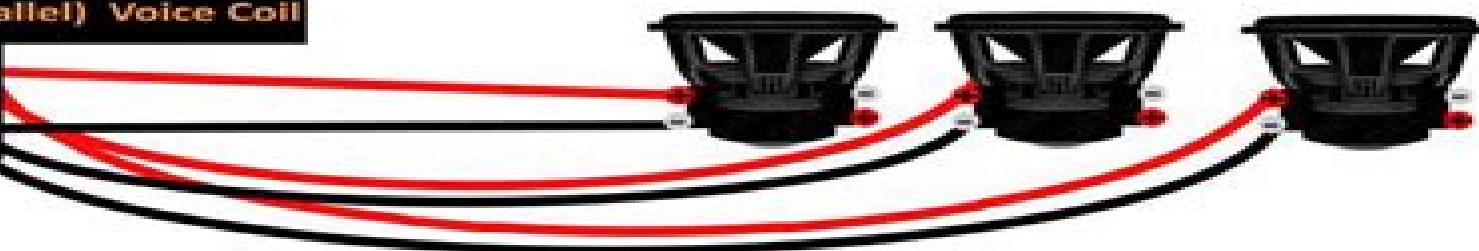
3 Sub, Single (Parallel) Voice Coil
