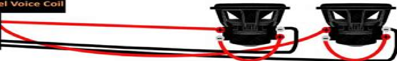
Dual Sub, Series - Parallel Voice Coil
