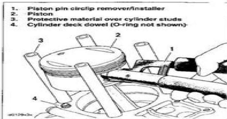
Figure 3-27. Piston Pin Circlip Removal (Part No. HD-42317)
