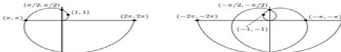
Figure 10.1.4 The spiral of Archimedes and the full graph of r = \theta .
