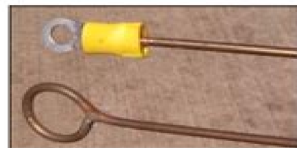
Fig 22.97 — Alternate methods for terminating element and radial tips on the simple groundplane antenna. See text. [Photo by KB9HJ]
