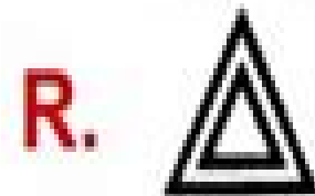
R. Emergency Flashers
