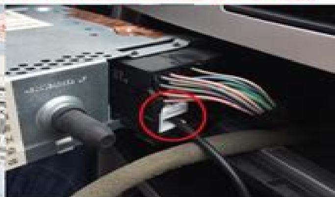
2. USING A U-SHAPED TOOL INSERT IT INTO THE MAIN UNIT REMOVAL HOLE
