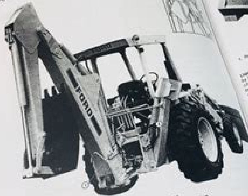
Figure 36 Backbone in Transport Position 1. Boom and Sling Transport Lock 2. Stabilizer Transport Chain 3. Extendable Dipstick Pinned and Lock
