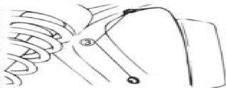
3. Loosen the screws ③ and remove the right frame cover.
