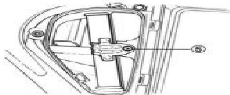
5. Loosen the screw ⑤ and remove the air cleaner element.
