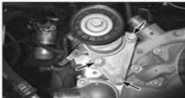
12.5a Main belt tensioner mounting bolts (V6 engine shown)
