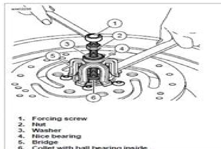
Figure 2-12. Removal Tool
