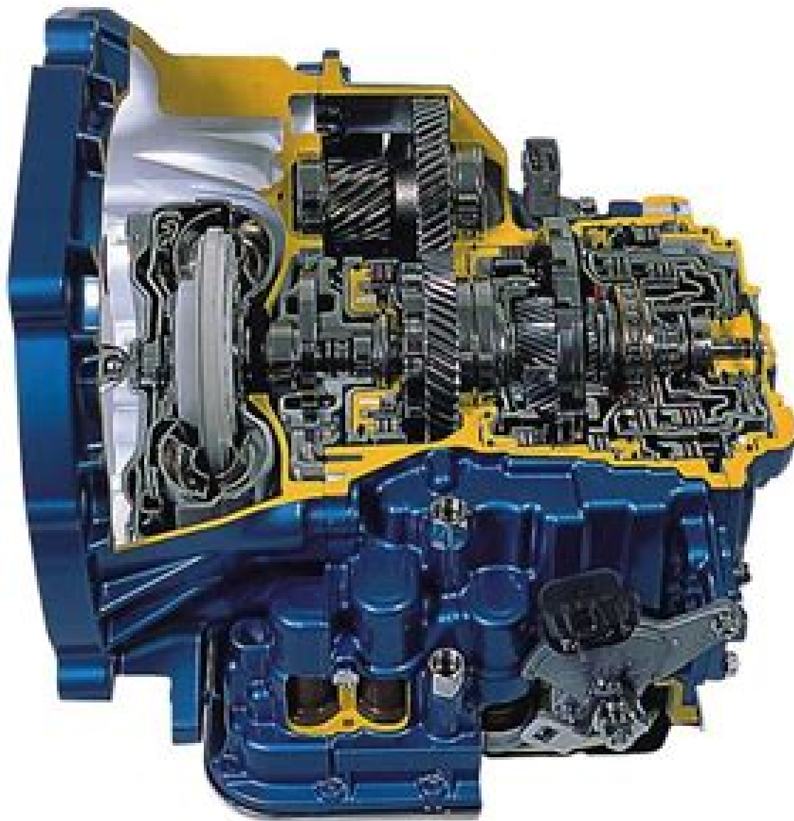
2010 GMDAT Aisin Warner 81-40LE ( MLQ ) Cutaway Four Speed FWD Automatic Transmission
