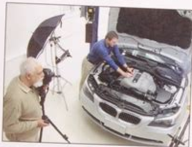
Bentley technical editors removing motor cover on V8 (N62) engine.
