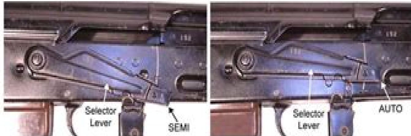
Figure 3. Selector Lever on SEMI (left) or AUTO (right).
