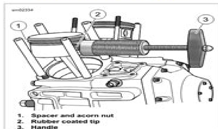
Figure 3-29. Piston Pin Remover (Part No. HD-42320-A)
