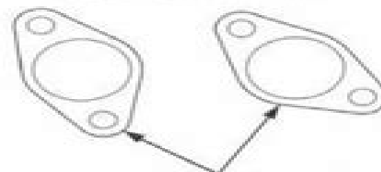
EXHAUST PIPE FLANGES
