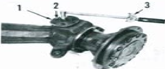
Fig. 8—Install special plate ACP-3080 (1) on upper king pin, then use a torque wrench (3) to measure torque required to turn planetary unit. Install shims on lower king pin only to adjust king pin bearing preload.
