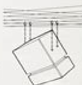
Figure 1. Suspended Studio Monitor Speaker System
