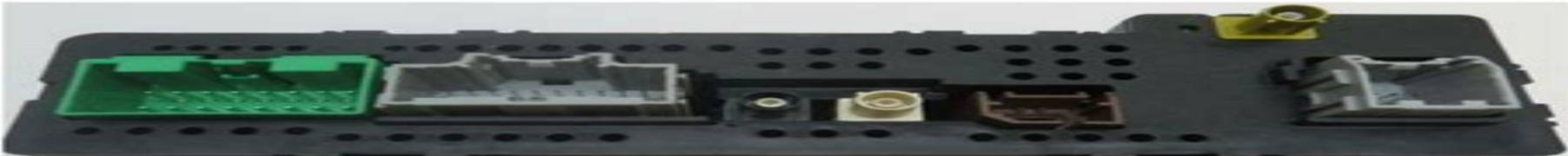
20 pin GM 13593932, 15491304 (15126710) Head Unit misc connector connector 8 pin GM 13591516 (19353873) connector p/n 84278530, 84361174, 84278524, 84361176, 84361178, 84361172
