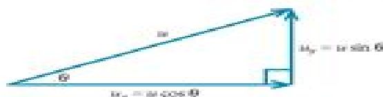
Figure 1.4 Breaking up the initial velocity ( u ) of a projectile into its vertical ( u_y ) and horizontal ( u_x ) components
