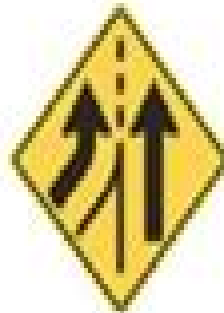
Added Lane sign
